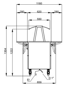
D = Drain El = Electrical inlet (power)
